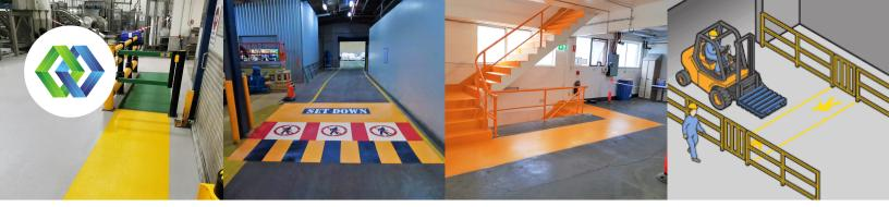
5. High visibility pedestrian barriers are installed in areas where forklifts are operating next to the path. Swing-in gates are also installed so that pedestrians can only enter the area after stopping to open the gate. This also means that in the situation where a pedestrian is in the forklift zone and needs to exit quickly, their route is intuitive and unimpeded by gates swinging conversely.
